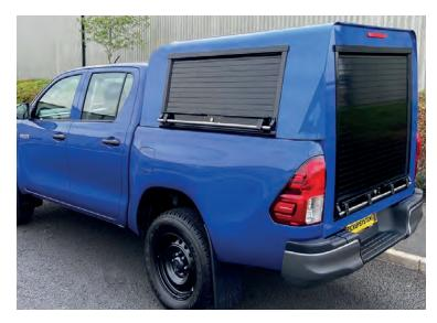
Constructed out of 9mm polypropylene plastic, our Easi-Tops aren't built using moulds, allowing them to easily be manufactured to fit a range of pick up vehicles.
